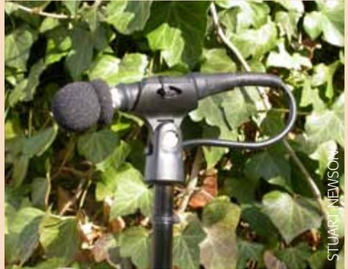
A microphone connected to a static detector is left out all night to automatically trigger and record every time a bat passes.
